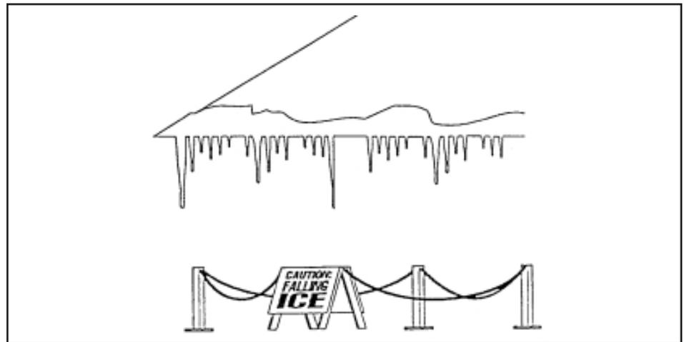
**Figure 3** Rope off areas where overhead ice is heavy or slides may occur.
