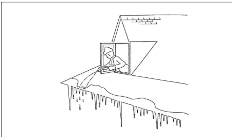
**Figure 4** Hot water being sprayed from dormer window
